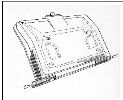
To remove back cover, slide the tabs as shown.
