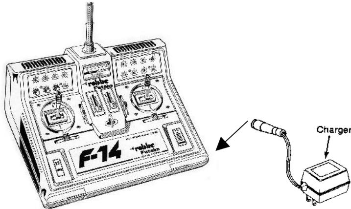
**Caution:** Do not overcharge the batteries as this could cause permanent damage to the transmitter batteries. (Doubling the normal charging time is the type of over charging that is meant here, and the battery getting hot.) When the battery level needle goes in the red, the robot should be turned off because the robot could act erratic without the transmitter signal.
